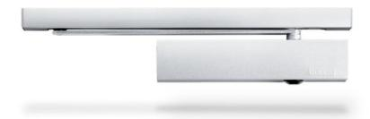
Overhead door closer with guide rail for single leaf doors of up to 1400 mm leaf width with latching action and brake-to-stop function with electric hold-open device
